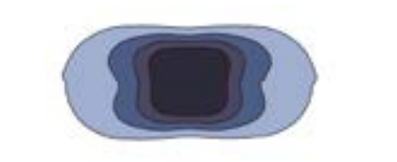
Symmetrical street optics - Medium beam L / H = 1,2
