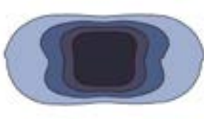
Symmetrical street optics - Medium beam L / H = 1,2
