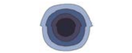
Rotosymmetrical road optics - Wide beam
