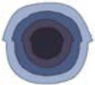
Rotosymmetrical road optics - Wide beam
