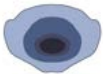
Asymmetrical optics - Very wide beam L / H = 1,5-2,0
