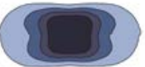
Symmetrical street optics - Medium beam L / H = 1,2
