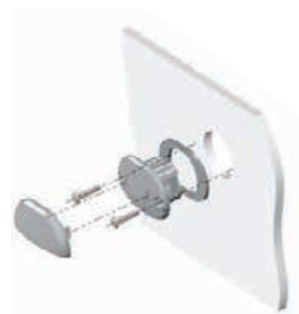
Mounting with screws. Push on plastic cap versions.
